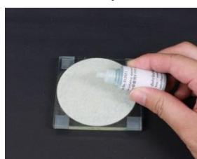
Paste the diamond polishing pad onto the glass plate. Then drip 2~3 drops of polishing diamond to the pad and add 2-3 drops of distilled water before polishing.
