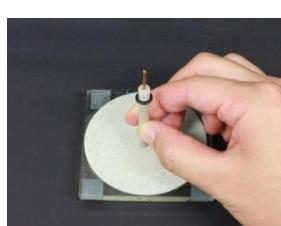
Press the electrode to the pad at right angle, and polish in motion of drawing 8 shape for few minutes under vertical state .
