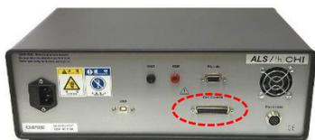
Figure 2-1 25-pin Cell Control terminal of ALS Model
