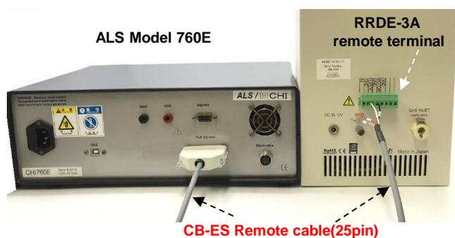
Figure 4-1 Remote connection of ALS Model and RRDE-3A
